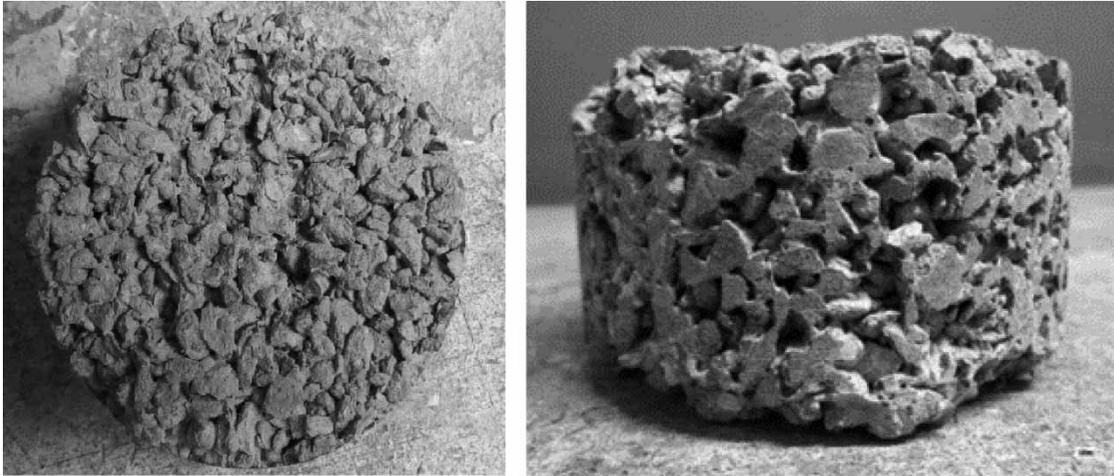
**Figure 2** | Permeable pavement used in the project.
