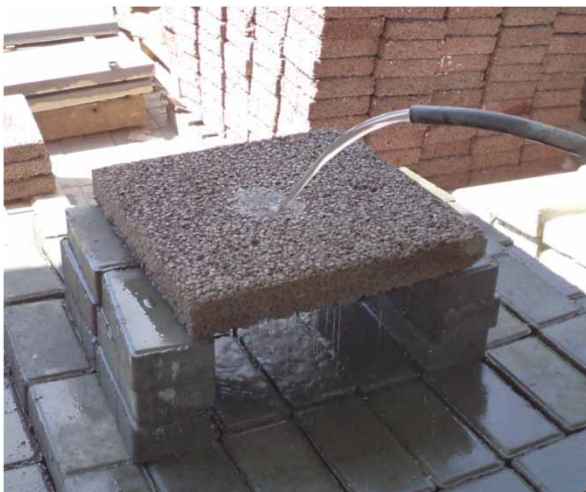
Figure 1 | Permeable pavement used in the project and image showing the infiltration in the pavement.
