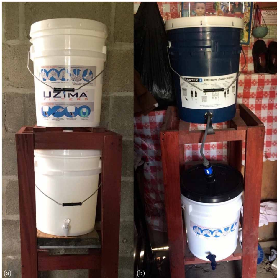
Figure 1 | (a) UZIMA water filter system and (b) Sawyer water filter system installed in households for the HOI hollow fiber filter program, Honduras, 2016–2017.
