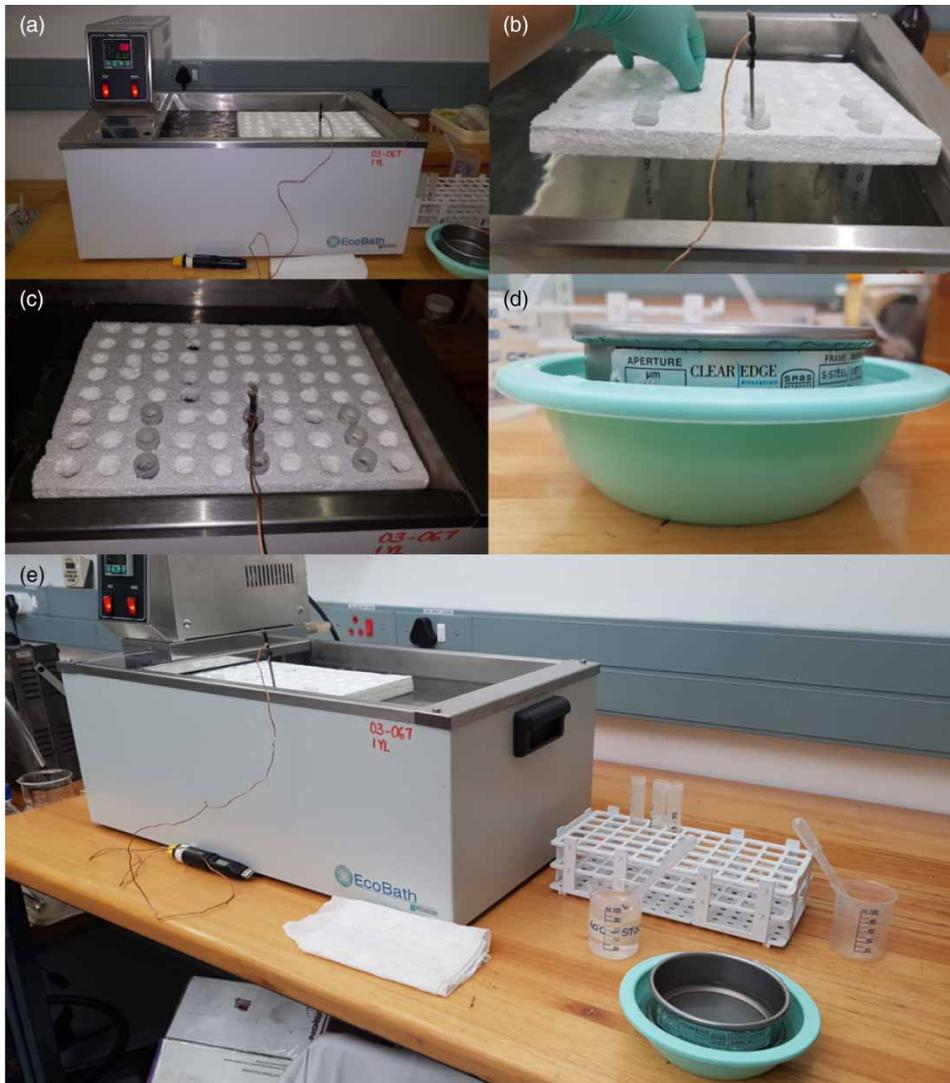
**Figure 1** | Experimental setup for heat treatment. (a) and (e) Preheated water bath with polystyrene racks containing test tubes and thermocouple. (b) and (c) Polystyrene rack setup with tubes containing water samples with spiked eggs in 15 mL plastic test tubes. (d) Sieve immersed in tap water, in plastic bowl.
