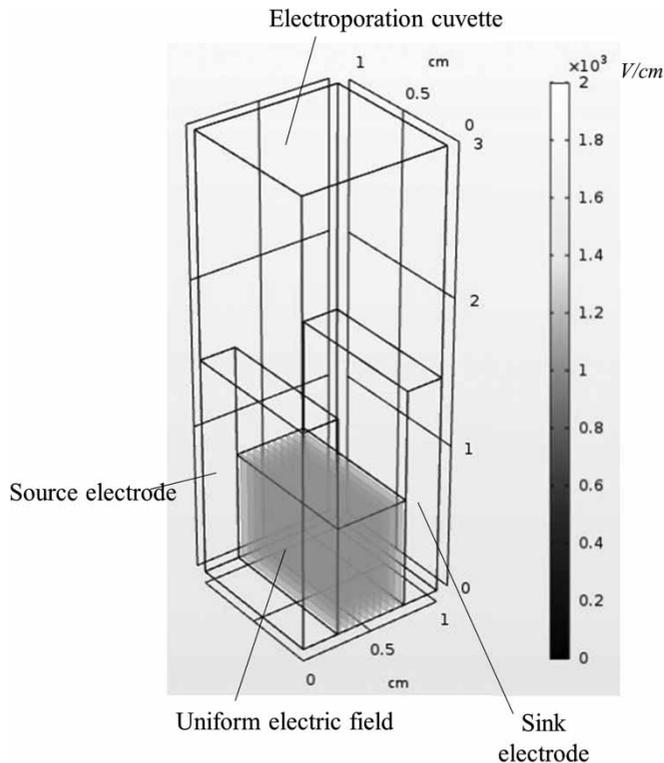
**Figure 1** | Illustration of the test cell cuvette used for *C. elegans* electroporation. The image includes the electric field uniformity at an applied potential of 500 V using COMSOL Multiphysics® modeling software.
