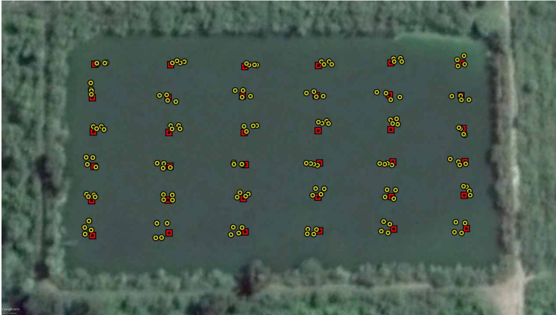
Figure 5 | Locations of WPs (squares) as planned in Mission Planner and the measurement points as registered by the GPS data logger (dots).
