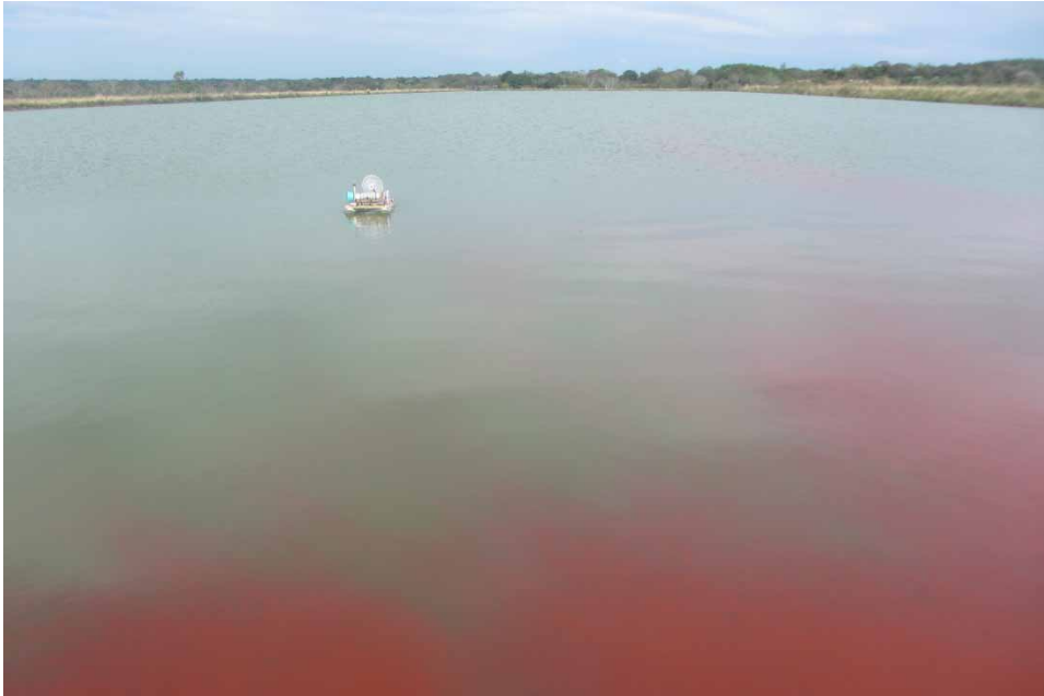
Figure 6 | Photo of the ASV during a Rhodamine WT tracer test in a WSP.
