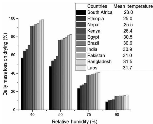
**Figure 3** | Daily mass loss on drying for the proposed breathable membrane toilet system predicted for ten developing countries over four ambient relative humidity conditions. Temperature in the legend is ten-year average temperature for each country.
