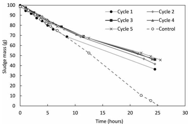
**Figure 2** | Sludge drying curve over five drying-and-reuse cycles. The first cycle control data is compared to five different faecal sludge cycles.
