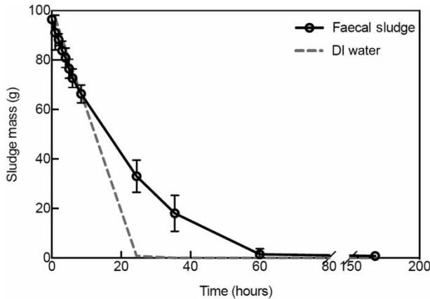
**Figure 1** | Drying of faecal sludge in new eVent laminate envelopes. Data points and error bars represent the average of triplicate envelopes and standard deviation, respectively.
