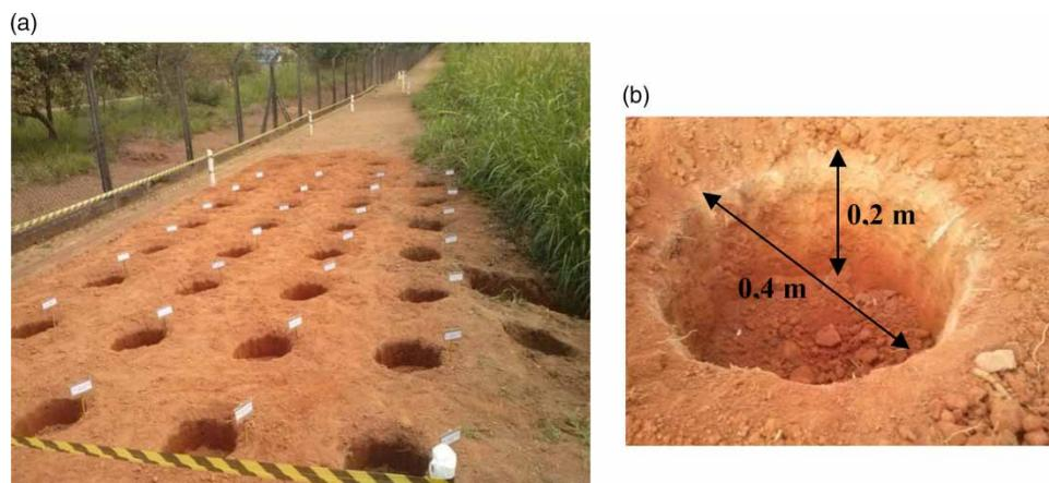
**Figure 2** | Panoramic view of the holes formed to fill with soil material mixed with organic residues collected from the VF-CW (a) and detail of the hole dimensions (b).
