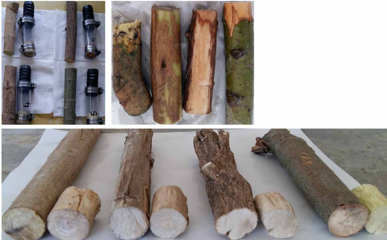
Figure 2 | Fresh wood (top left), wet preserved wood (top right) and dry preserved wood (bottom); Combretum erythrophyllum , Tarchonanthus camphoratus , Leonotis leonurus and Salix mucronata left to right, respectively.
