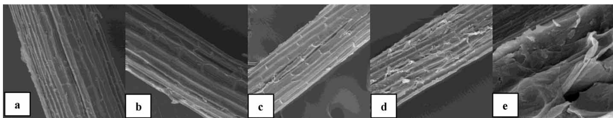
Figure 1 | Scanning electronic microscopy images of sisal fibers: (a) without any treatment ( \times 200 ); (b) after solubility assays in hydrochloric acid ( \times 200 ); (c) after solubility assays in sodium hydroxide ( \times 200 ); (d) after 2 months of the filter's operation ( \times 200 ); and (e) after 2 months of the filter's operation ( \times 2000 ).
