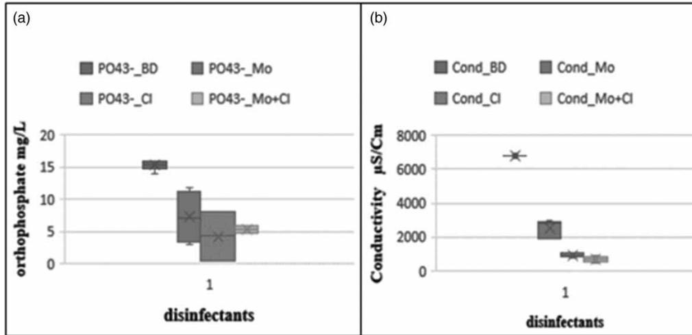
Figure 5 | Variation of orthophosphate (a) and electrical conductivity (b).
