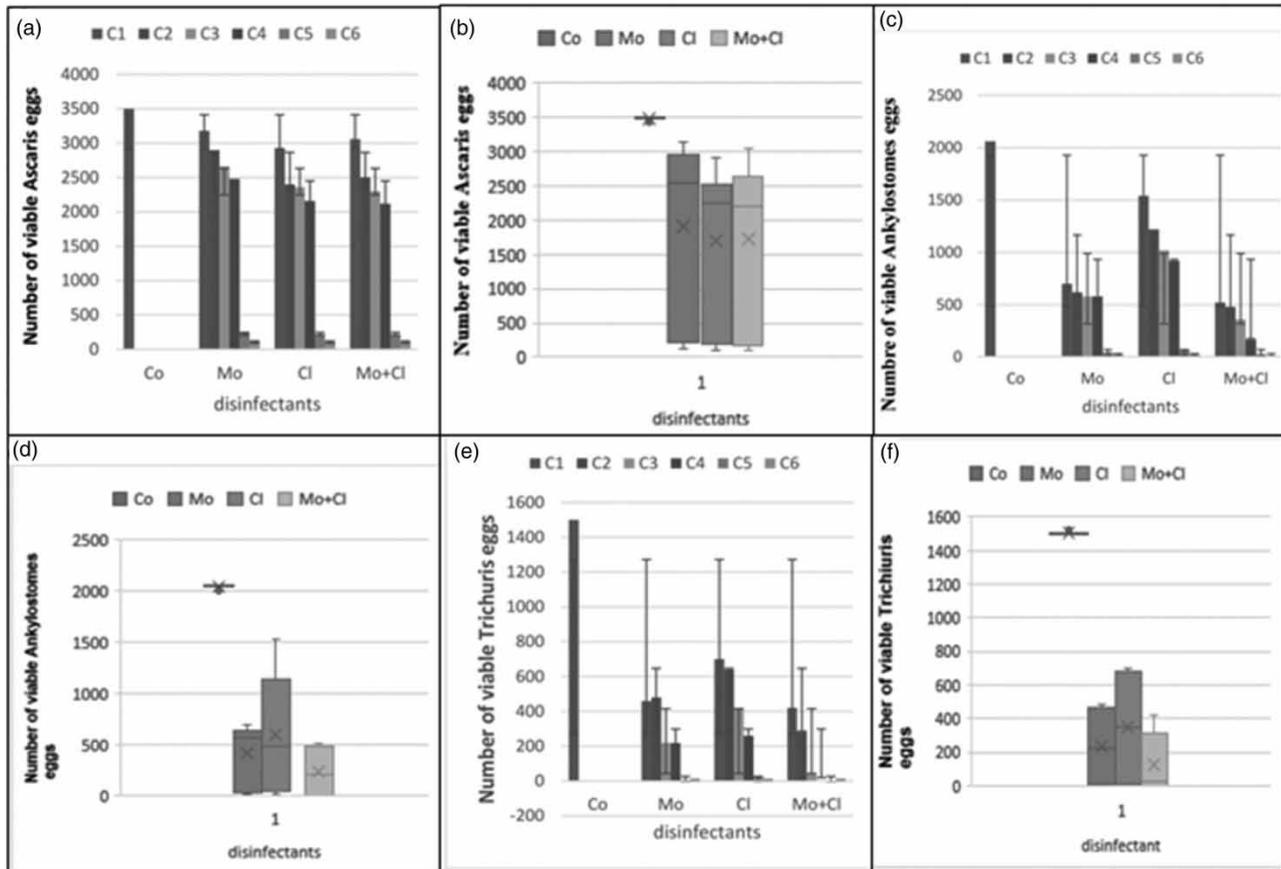
**Figure 2** | Change in the number of eggs of *Ascaris*, *Ankylostoma* and *Trichuris* based on the different concentrations of disinfectants used. Co: control; Mo: *Moringa*; Cl: calcium hypochlorite; Mo+Cl: *Moringa* associated with chlorine.
