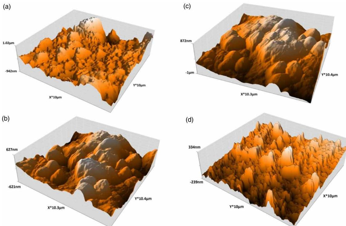
**Figure 5** | Atomic force microscopy 3-dimensional images of 30-day biofilm of *L. pneumophila* sg 2–15 grown on galvanized steel (a) and (b) and PVC (c) and (d) after (a) and (c) and before (b) and (d) chlorination.
