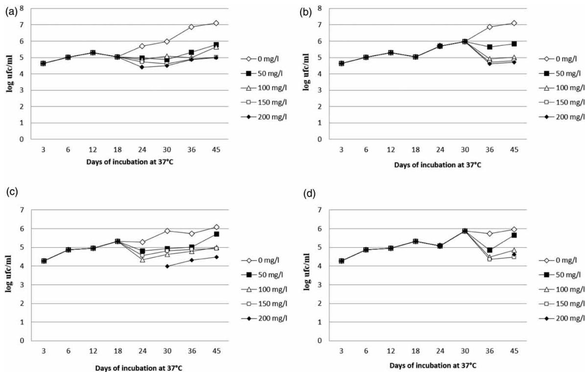
**Figure 4** | The growth of *L. pneumophila* sg 2-15 on galvanized steel (a) and (b) and PVC (c) and (d) when challenged with a range of concentrations of chlorine at day 18 (a) and (c) and day 30 (b) and (d).
