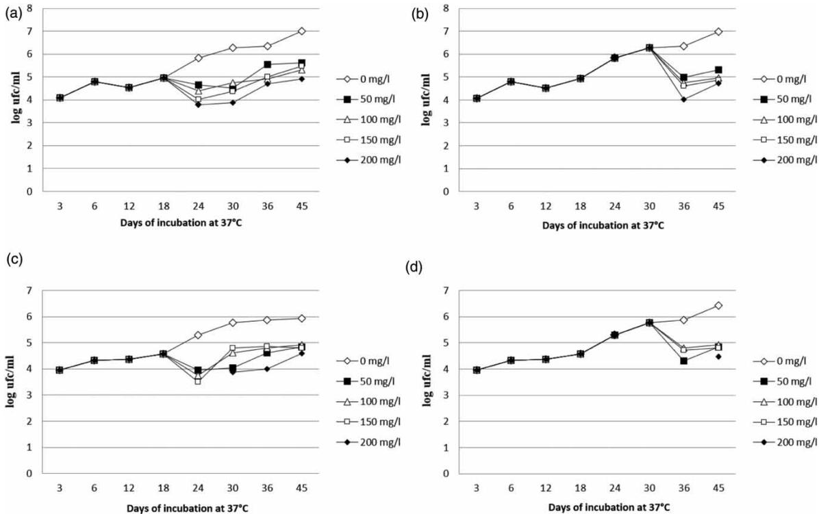
**Figure 3** | The growth of *L. pneumophila* sg 1 on galvanized steel (a) and (b) and PVC (c) and (d) when challenged with a range of concentrations of chlorine at day 18 (a) and (c) and day 30 (b) and (d).
