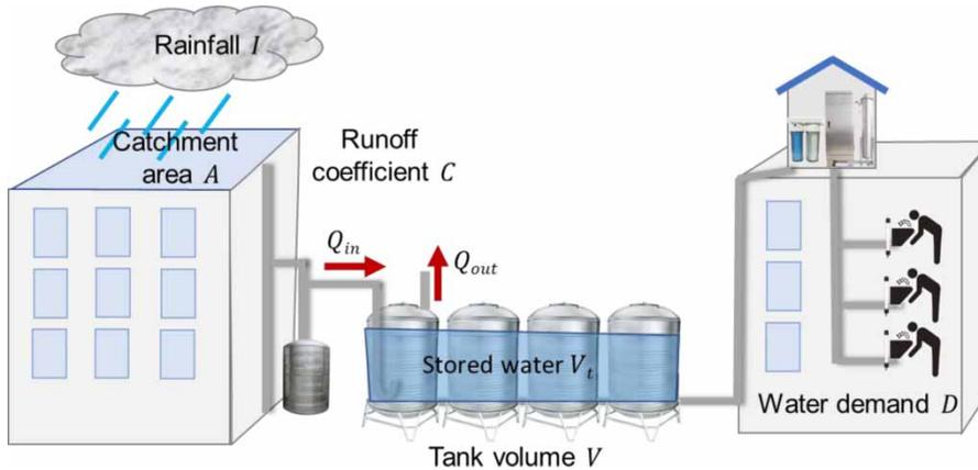
Figure 5 | Schematic diagram of the RFD at Ly Nhan HCF.
