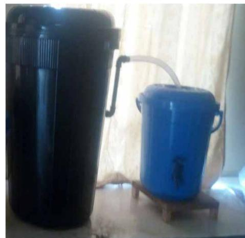
**Figure 8** | Biosand water filters system.
