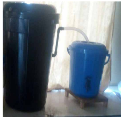
Figure 8 | Biosand water filters system.
