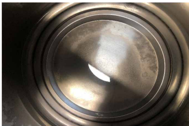
Figure 7 | Mineral salt deposition inside the water compartment of a kettle.
