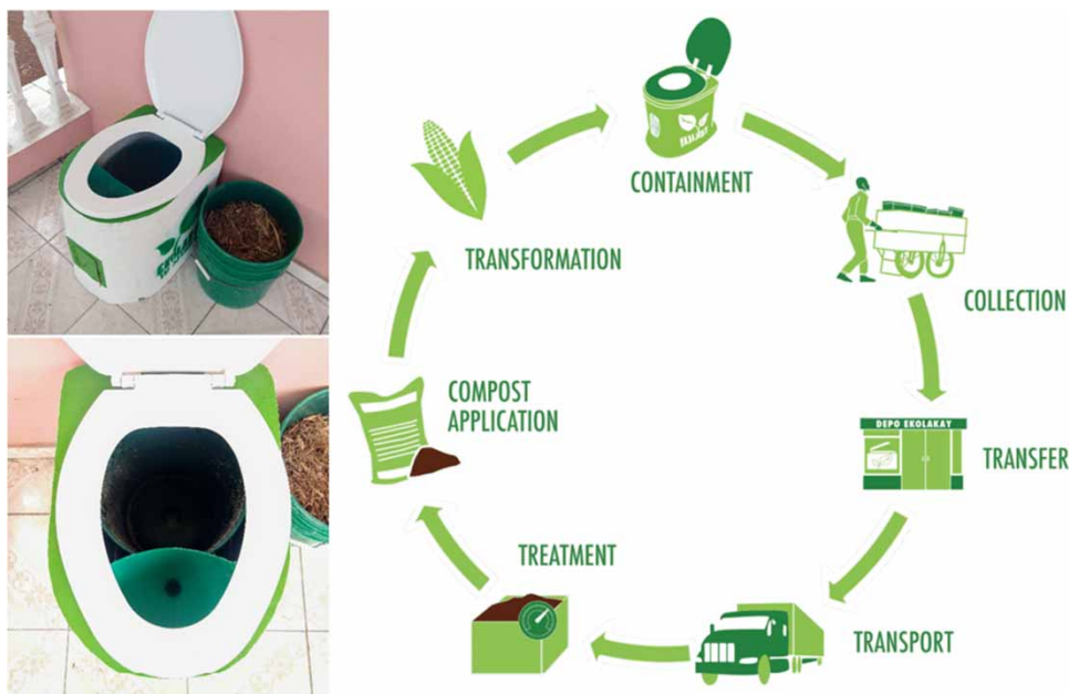
Figure 1 | EkoLakay toilet technology and the CBS sanitation resource chain (Photographs by FV; Graphics used with permission of SOIL). Please refer to the online version of this paper to see this figure in colour: http://dx.doi.10.2166/washdev.2021.162 .
