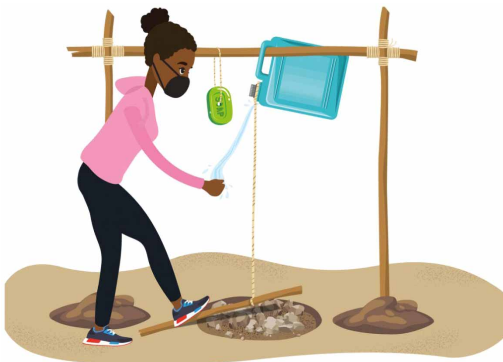
Figure 2 | Tippy-tap schema. Credit: UNICEF.
