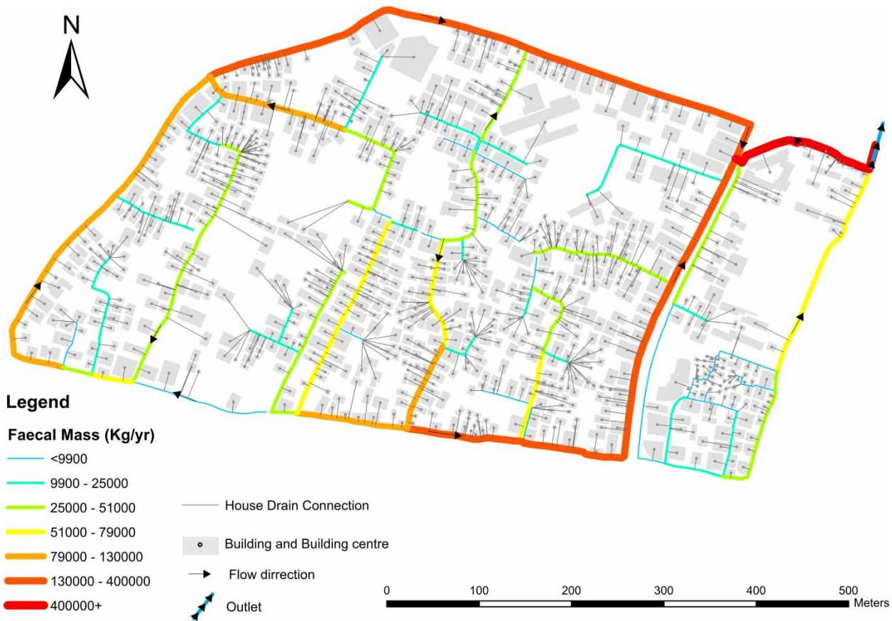
Figure 4 | Sankey representation of faecal movement. The discharge point, i.e., outlet of the catchment is located in the top of the northeast corner, which is carrying 810 tonnes of faecal mass on a yearly basis. The values were categorised using Jenks natural breaks (with two significant digits rounding) as mentioned in the 'Methods' section.
