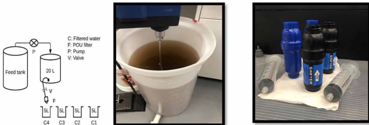
Figure 1 | POU filtration system setup (left), mixing of synthetic water in feed tank (center), membrane filters, and backwash syringes (right).
