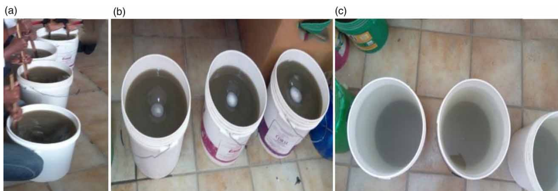
Figure 1 | (a) Rapid mixing after coagulation with different dosages of dCSE (coagulation process), (b) slow self-water mixing (flocculation processes) and (c) treated water during the settling process.
