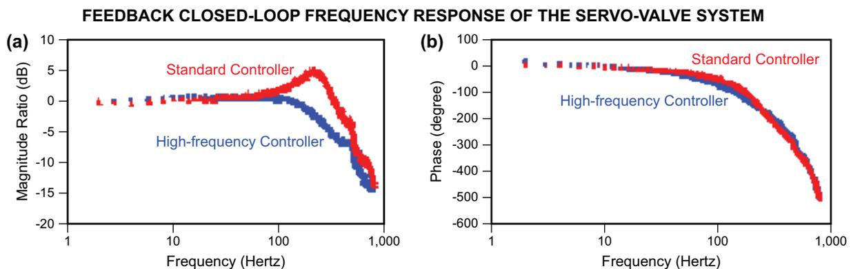
**Figure 6: Servo-valve closed-loop frequency response: (a) magnitude ratio plot, (b) phase plot. The servo-valve closed-loop frequency response of a standard controller is compared with that of the new high-frequency controller. The high-frequency controller offers advantages in suppressing significant resonances at 200 and 450 Hz. With dampened resonances, a smooth servo-valve system dynamic response is achieved.**
