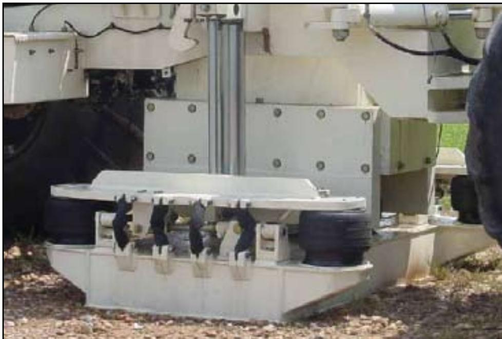
**Figure 7: The vibrator is on a gravel track in Sealy, Texas, USA. The gravel track is about 25.4 cm thick and overlies Texas black clay. The gravel track is fairly flat and the vibrator is well-coupled with the ground surface.**
