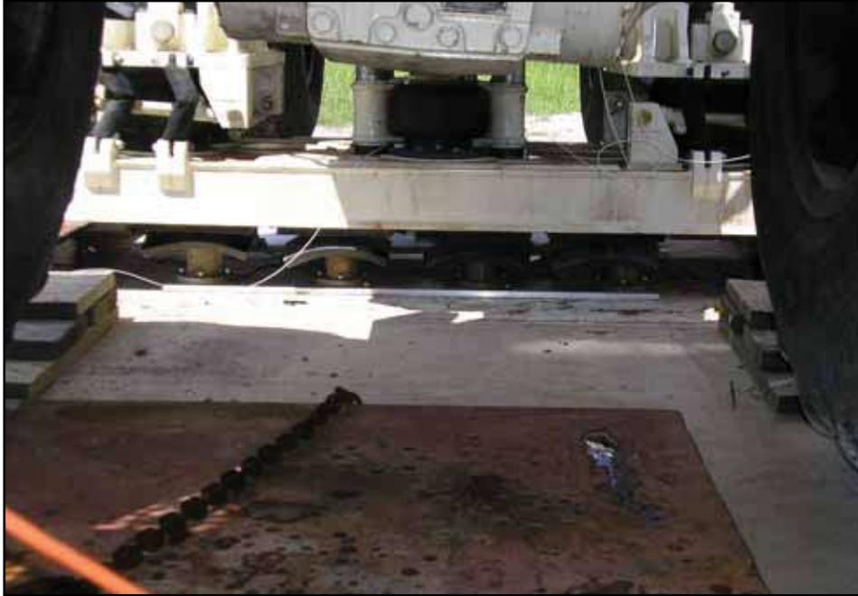
Figure 11: The vibrator is on load cells in Sealy, Texas, USA. A total of eight load cells were mounted on the concrete and evenly distributed beneath the baseplate. Two small rubber pads were placed on top of each load cell to protect it from metal-to-metal contact. Under this loading condition, the baseplate was well-coupled with load cells but the contact area was small. The flexural vibration and complex rocking of the baseplate were severe.
