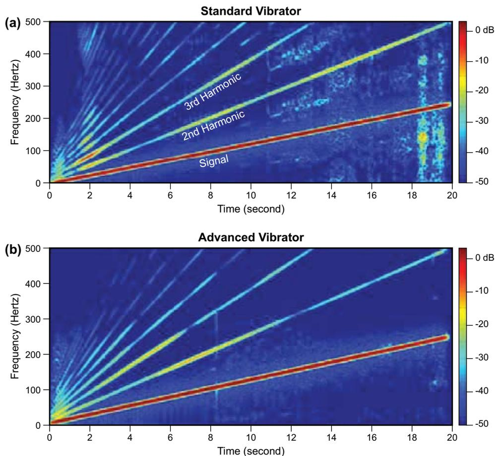
**Figure 13: Frequency-time representation of the weighted-sum ground force on a gravel track in Waller, Texas; (a) Standard AHV-IV vibrator; and (b) AHV-IV vibrator with the new mass and baseplate system.**
