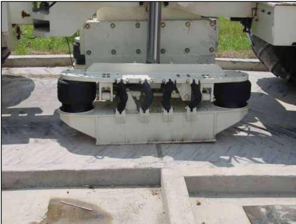
**Figure 9:** The vibrator is on concrete in Sealy, Texas, USA. The baseplate was placed partially on flat concrete and partially on a ramp with an air gap between a section of the baseplate and the ground. The purpose was to create an uneven loading so that complex rocking motions would be generated during vibration.
