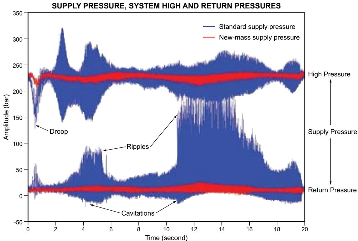
**Figure 3: Comparison of the standard supply pressure (blue) and the new-mass supply pressure (red) on ION's AHV-IV vibrator performing a 1 to 201 Hz linear sweep in 20 seconds. The new design dramatically reduced pressure ripples in both system high and return pressures. Cavitations in the system return pressure and the 'droop' at low frequencies in the system high pressure were eliminated.**
