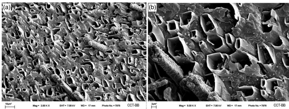
**Figure 4** | SEM image of PPy/Cu-covered steel electrode after being used in a 5 h disinfection process at  $Re = 115$ . The PPy film was formed potentiostatically at 0.80 V during 10 min in a solution containing 0.25 M Py + 0.50 M NaSa. The copper immobilization was obtained by immersion in 0.10 M  $CuSO_4 + 0.10$  M  $Na_2SO_4$  solution of pH 1 under OCP conditions during 24 h. Magnifications: (a) 2,000 $\times$  and (b) 5,000 $\times$ .
