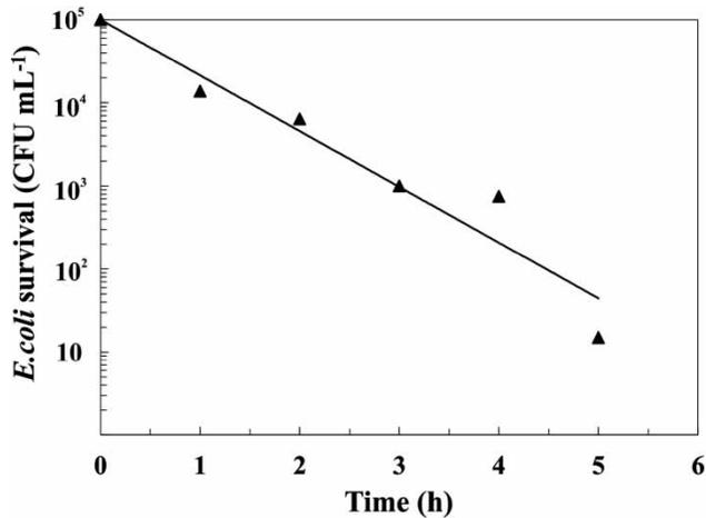
**Figure 6** | Bactericidal activity of re-charged PPy/Cu modified electrodes against *E. coli* in 100 mL of well water recirculating at  $Re = 115$ . Full line corresponds to the exponential fitting of the experimental data.
