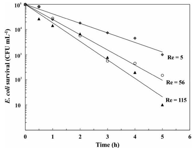
**Figure 2** | Bactericidal activity for PPy/Cu-covered electrodes against *E. coli* in 100 mL of well water recirculating at different Re numbers. The full lines correspond to the exponential fitting of the experimental data. The standard deviation associated to the experimental data is no larger than 25%.
