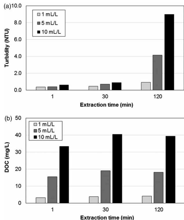
**Figure 8** | Turbidity (a) and DOC (b) with adding the MO seed extract by extraction time to distilled water (Extraction condition: 5 g MO/100 mL, Extract dose: 1, 5, and 10 mL/L, Extraction time: 1, 30, and 120 min).
