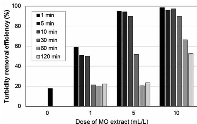
**Figure 2** | Turbidity removal efficiency in coagulation test using MO seed extract made by various extraction time (Extraction condition: 5 g MO/100 mL, 100 rpm, 1–120 min, Dose of MO extract: 1–10 mL/L).
