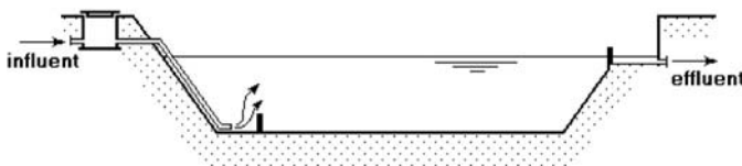
Figure 4.6. Schematic representation of an anaerobic pond
