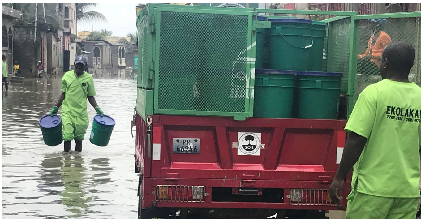
Figure 9: With small, sealed waste containers that are frequently collected, container-based services minimize the risk of waste release into the environment—even during flooding—and are more likely to be able to continue to operate during adverse conditions (Image source: SOIL).
