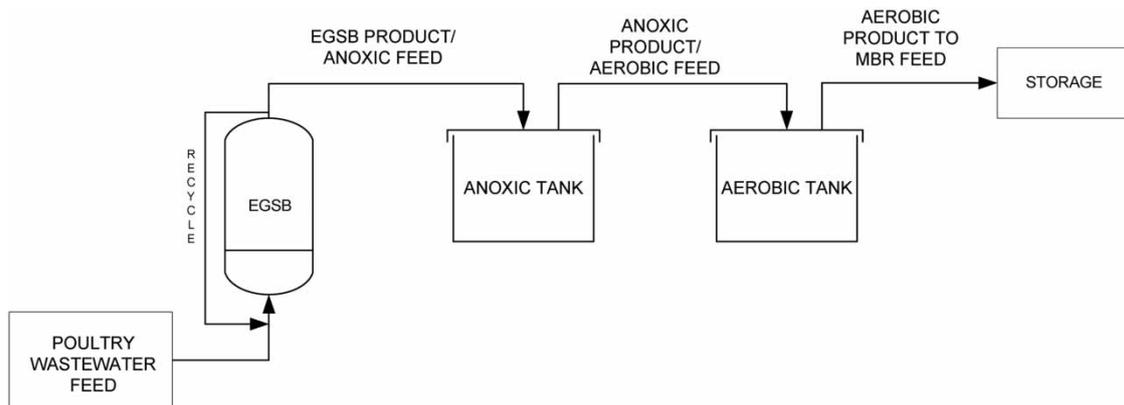
**Figure 1** | Schematic diagram for the laboratory bench-scale EGSB, anoxic and aerobic bioreactor system.
