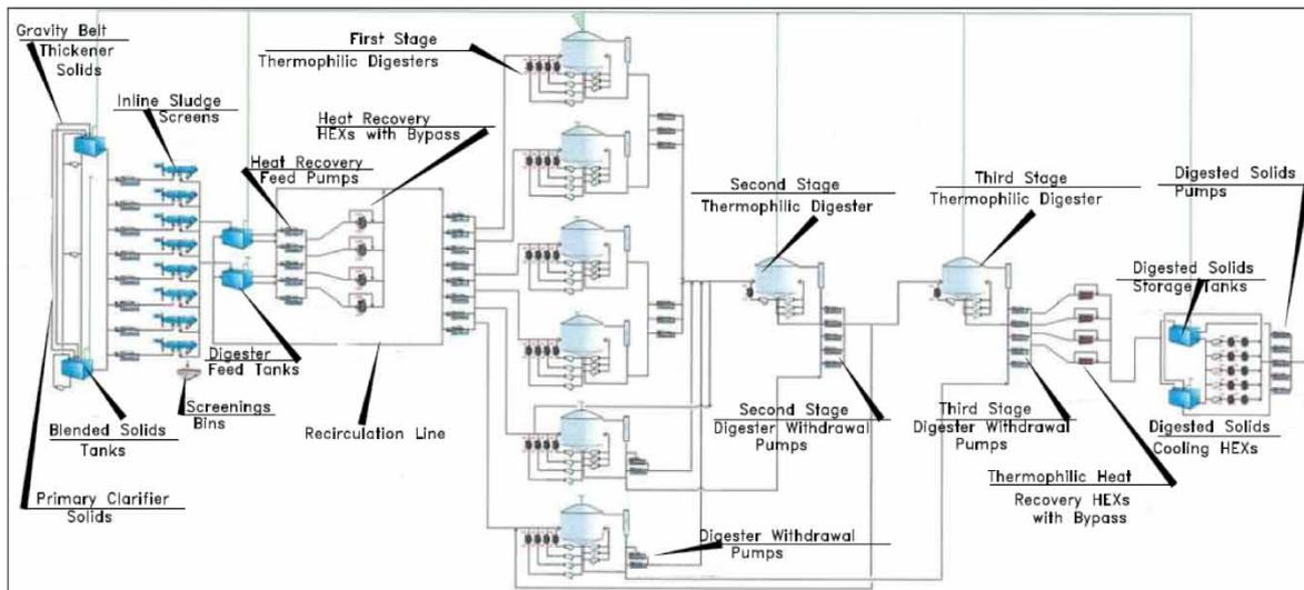
**Figure 11** | Anaerobic Digestion Facility Process Flow Diagram.
