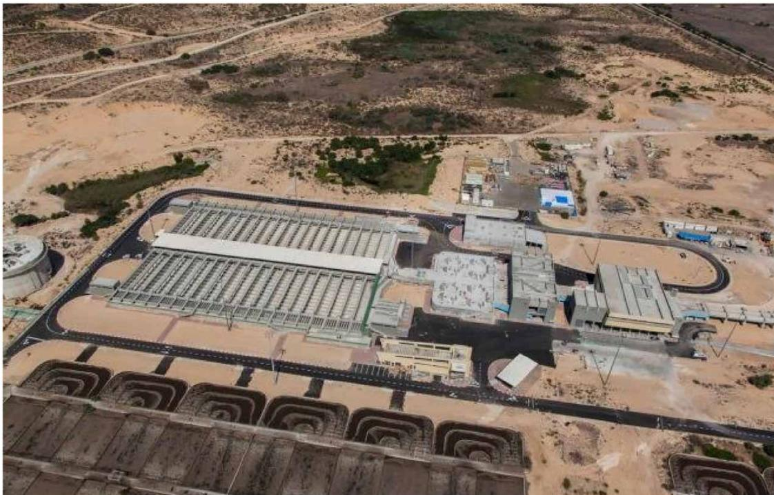
**Figure 6** | SHAFDAN new headworks and primary clarifiers.
