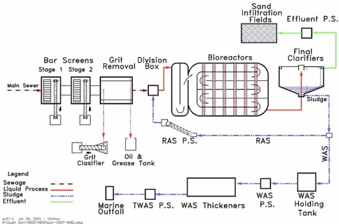
**Figure 1** | SHAFDAN current process flow diagram.
