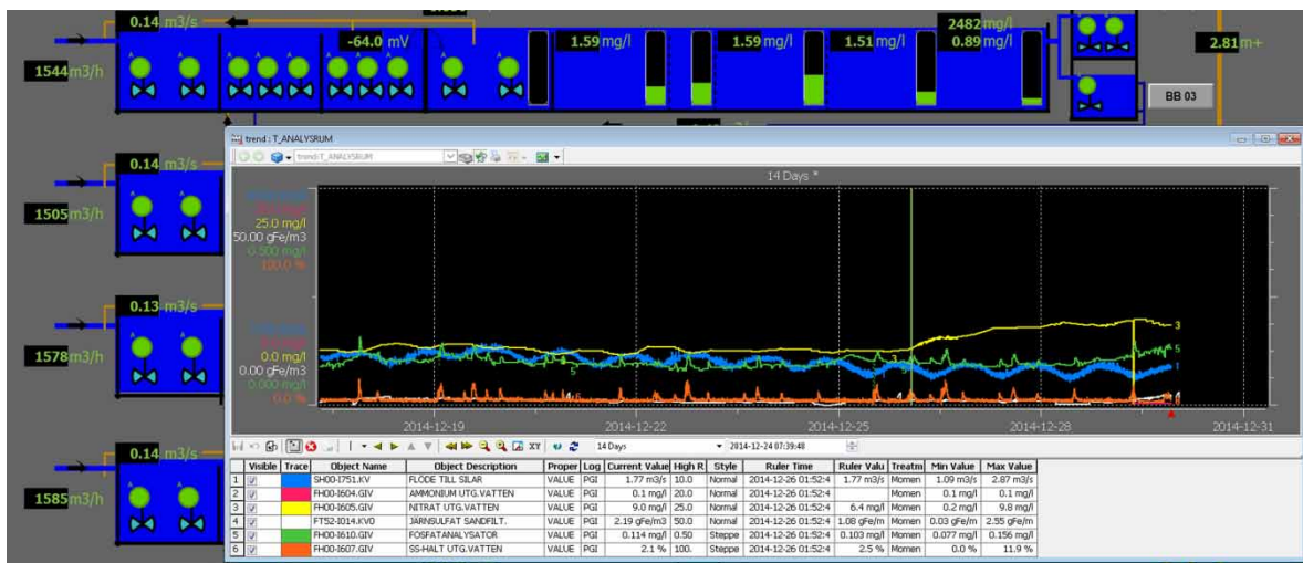
Figure 2 | Example of the DCS 800xA 5.1 controlling all equipment at the Kåppala WWTP and surrounding facilities.
