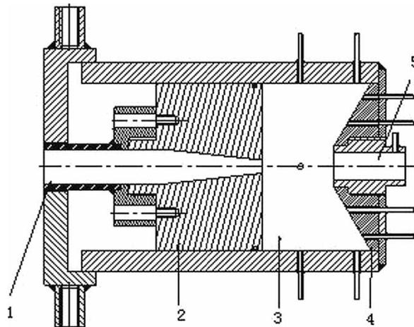
**Figure 2** | Structure of a self-excited pulsed jet device. 1- Water inlet, 2- top nozzle, 3- self-excited oscillation cavity, 4- diffuser section, and 5- bottom nozzle.
