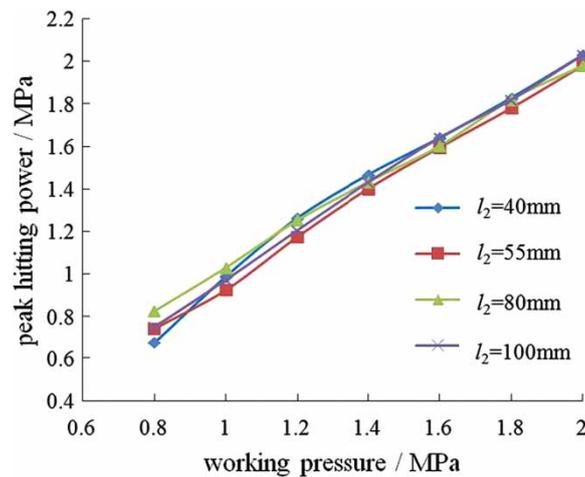
**Figure 6** | Pulsed jet peak hitting power corresponding to different bottom nozzle lengths.
