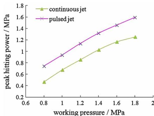
**Figure 9** | Peak hitting power curves for pulsed and continuous jets.
