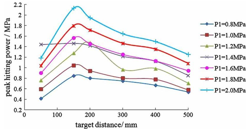
**Figure 8** | Peak hitting power corresponding to different target distances.
