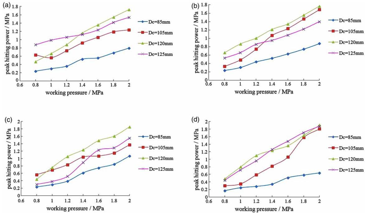
**Figure 4** | Peak hitting power corresponding to different cavity diameters,  $L_c$ : (a) 45 mm, (b) 60 mm, (c) 75 mm, and (d) 90 mm.
