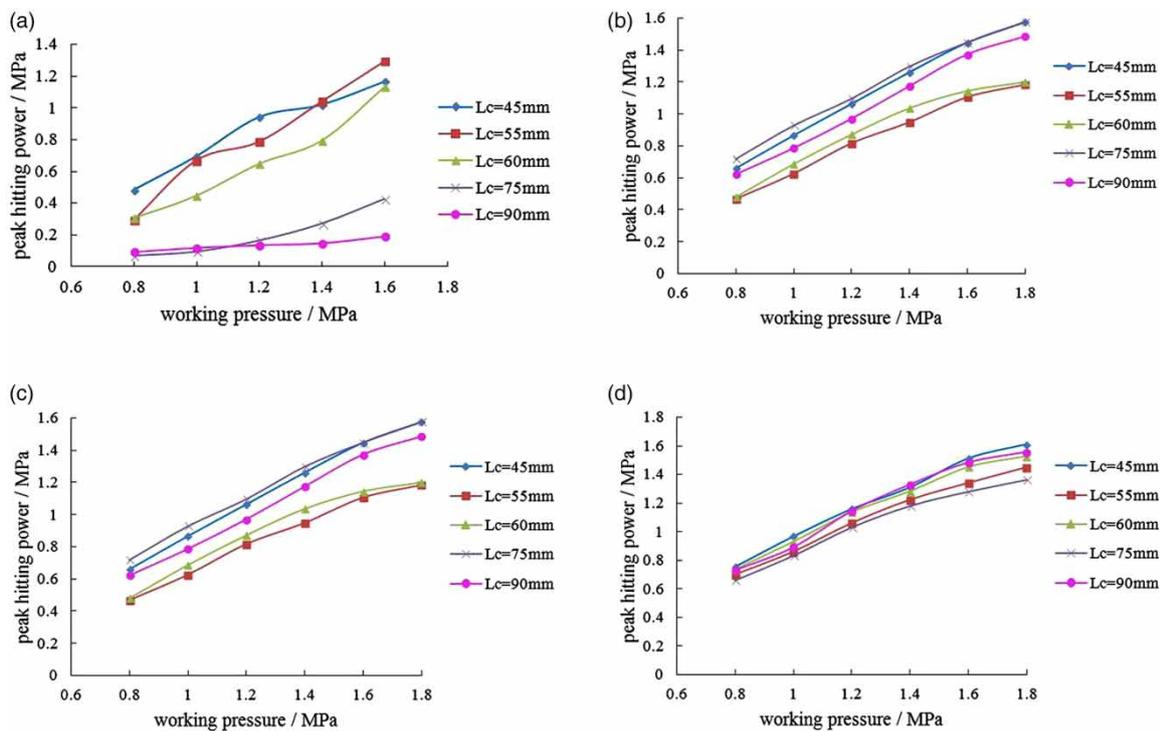
**Figure 3** | Peak hitting power corresponding to different cavity lengths,  $d_2$ : (a) 14 mm, (b) 16 mm, (c) 18 mm, and (d) 20 mm.
