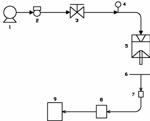
**Figure 1** | Self-excited pulsed jet test setup. 1- Multistage centrifugal pump, 2- electromagnetic flowmeter, 3- gate valve, 4- pressure gage, 5- self-excited pulsed jet device, 6- target plate, 7- pressure transducer, 8- data acquisition system, and 9- computer.
