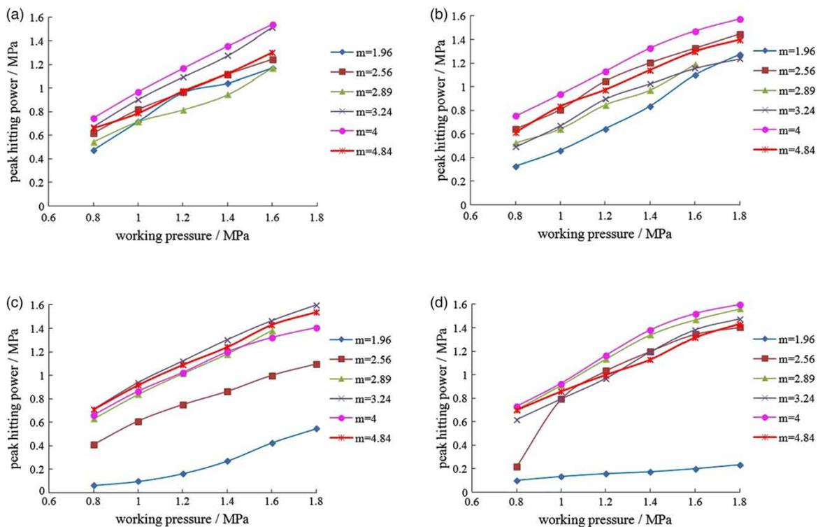
**Figure 5** | Peak hitting power corresponding to different bottom/top nozzle areal ratios, with different oscillation cavity lengths,  $L_c$ : (a) 45 mm, (b) 60 mm, (c) 75 mm, and (d) 90 mm.
