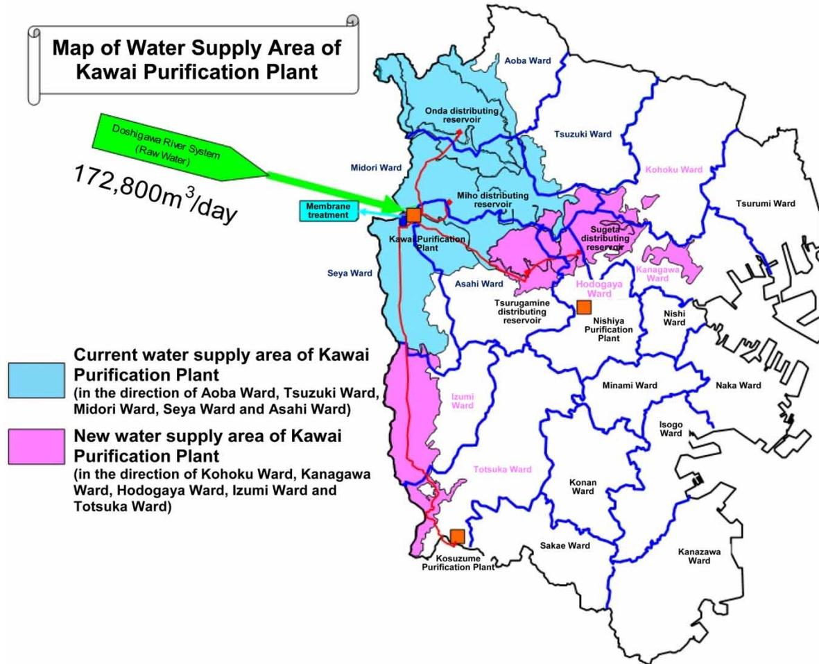
**Figure 6** | Water supply area of the Kawai Purification Plant (blue denotes the area prior to build-up, and pink denotes the added area after build-up).
