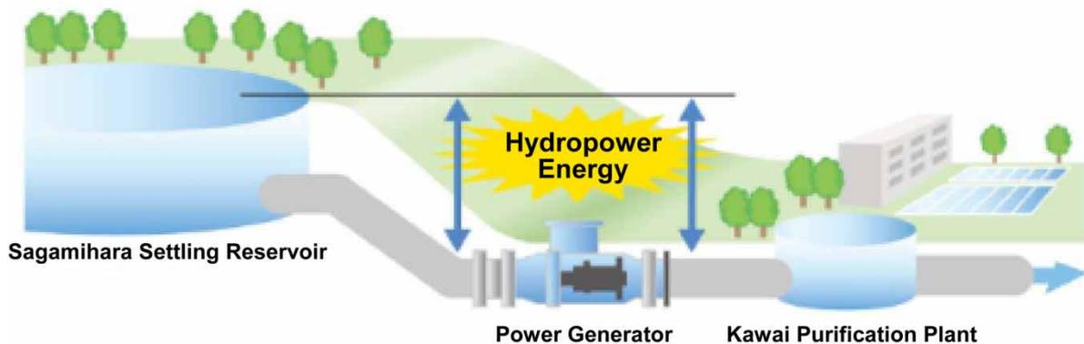
**Figure 4** | An image of the micro hydropower generation system at the Kawai Purification Plant.
