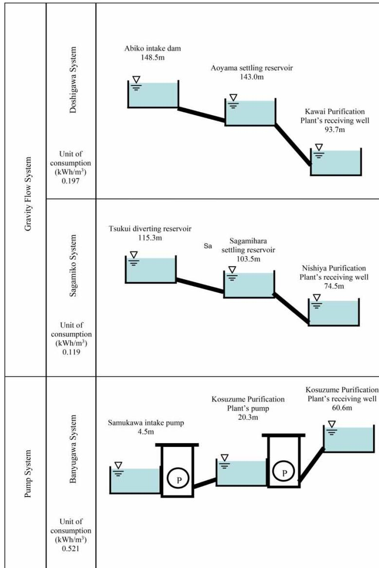
**Figure 5** | Elevation and units of consumption of facilities by individual water source system (Units of consumption from Yokohama Water Works Bureau's annual power report of FY2013).
