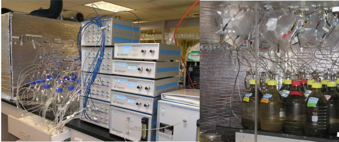
**Figure 1** | On-line respirometer and digester bottles.
