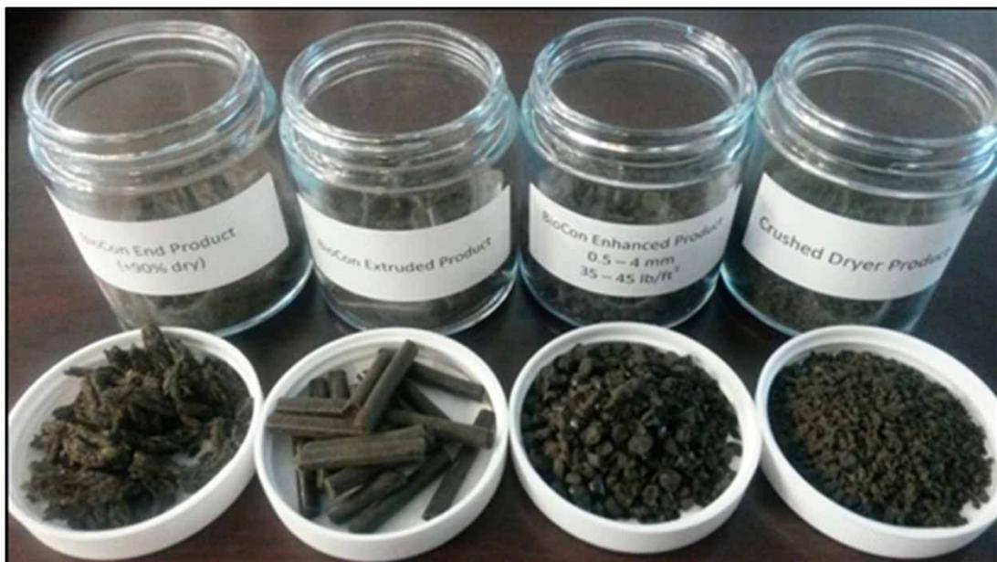
**Figure 6** | The Belt B dryer products – left to right: dried/non-pelletized, dried/pelletized/not cut, dried/pelletized/cut, and dried/non-pelletized/crushed.
