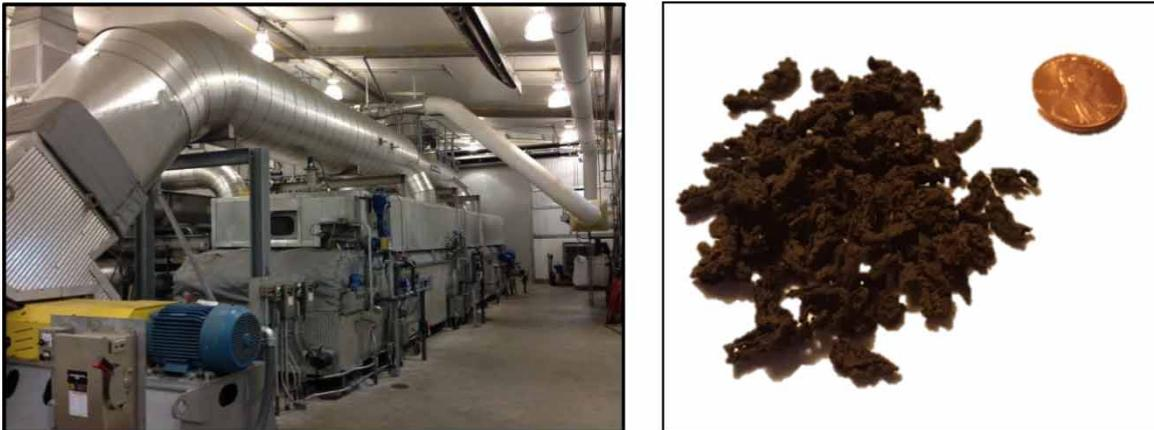
**Figure 5** | Single pass belt dryer – i.e., no recirculation – and typical product.
