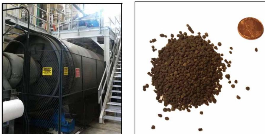
**Figure 4** | Drum dryer and typical product.
