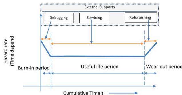
Figure 2 | Types of external supports.
