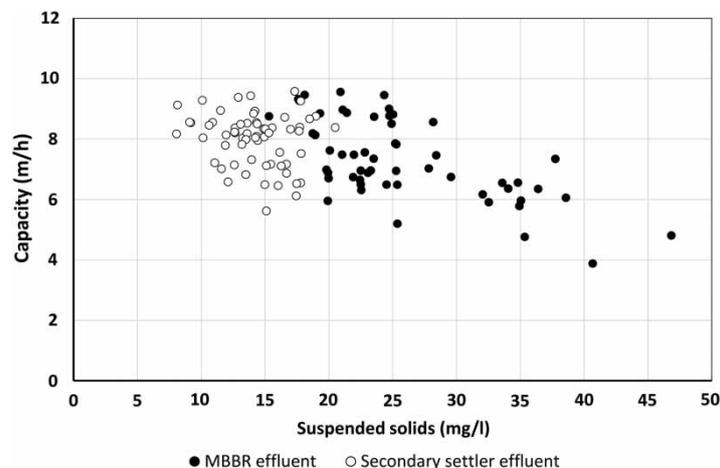
**Figure 5** | Hydraulic capacity versus SS concentration (Nov 2012–May 2013). Data corresponds to occasions when the flow from the secondary settler and MBBR made up at least 60% of the total flow.
