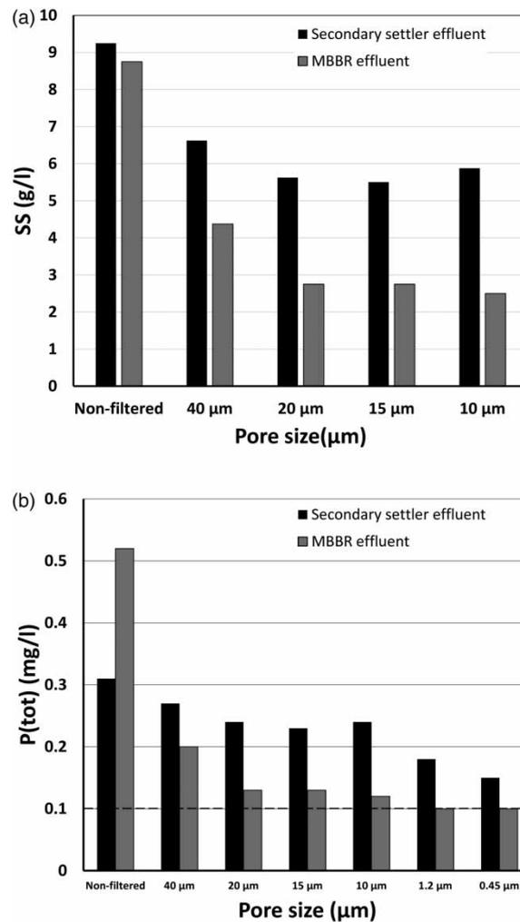
**Figure 4** | Concentration of (a) SS and (b) P<sub>tot</sub> in different fractions of the MBBR, secondary settler and disc filter effluents.
