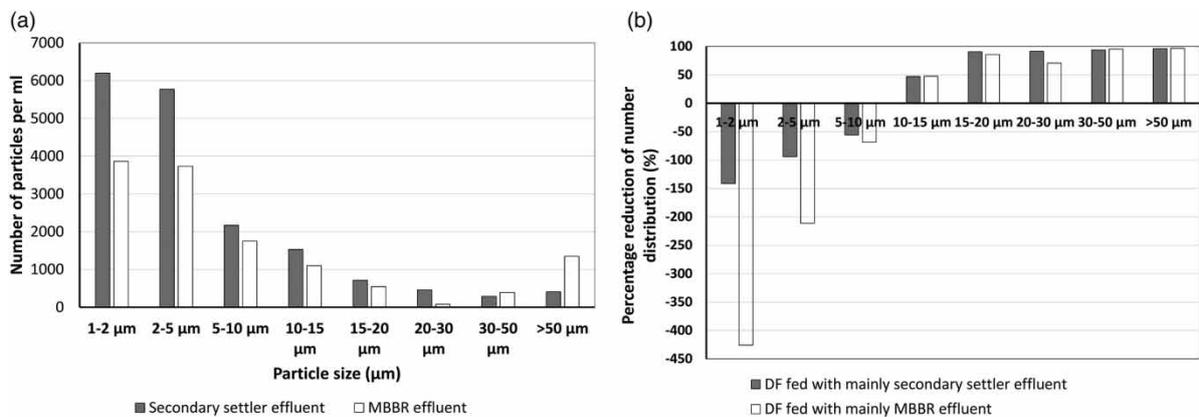
**Figure 3** | Particle size analysis of MBBR and secondary settler effluent (a) number size distribution, and (b) percentage reduction in number of particles of different sizes.
