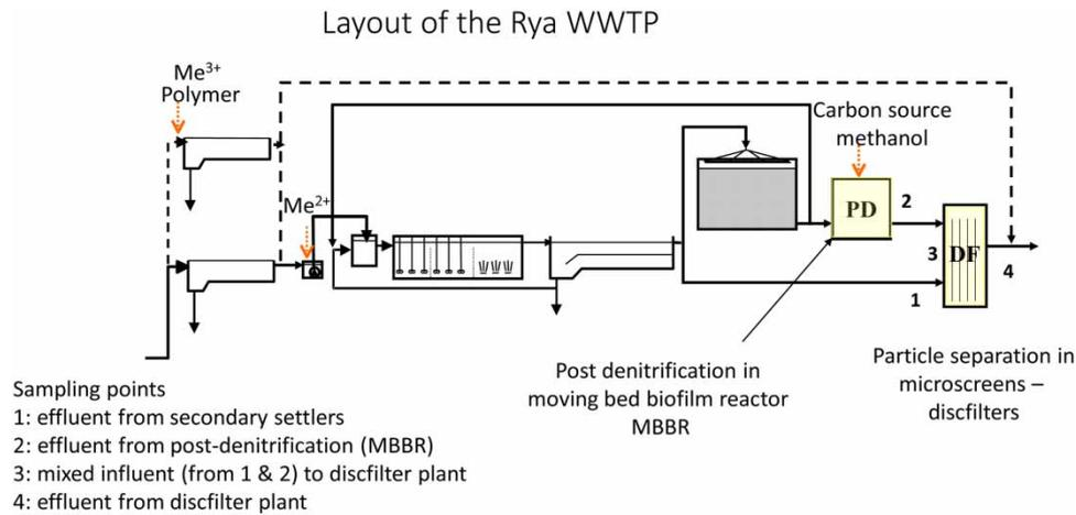
**Figure 1** | Process layout of the Rya WWTP.
