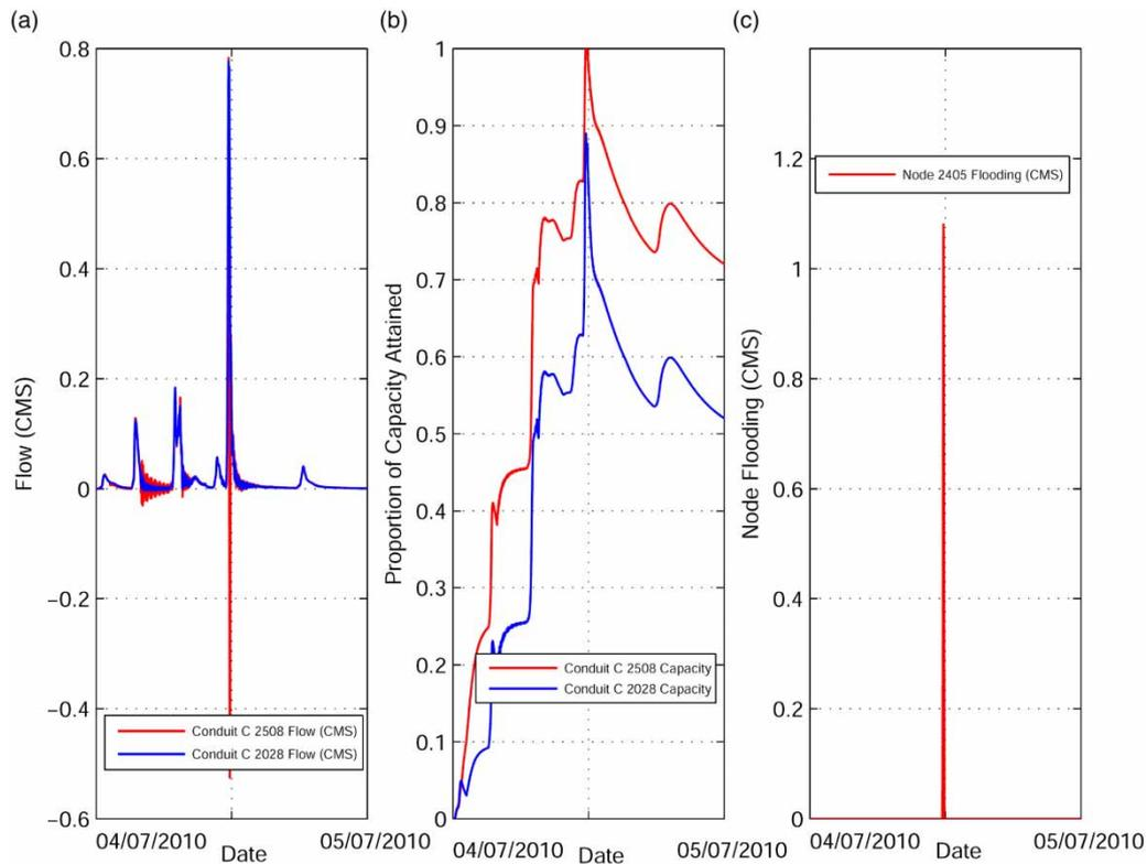
**Figure 6** | SWMM simulation results (a) Conduit flows, (b) Conduit capacity and (c) Node flooding.
