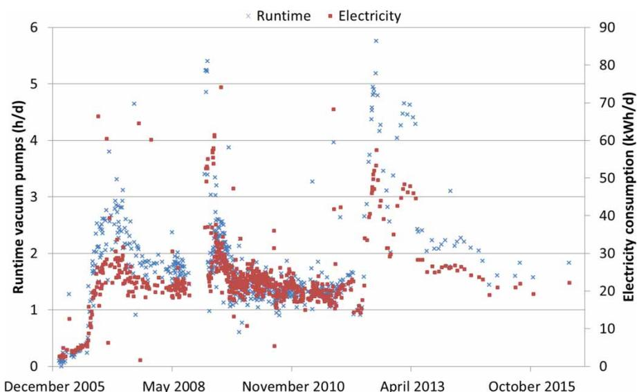
**Figure 4** | Vacuum pump runtime (blue crosses) and electricity consumption (red dots) for the vacuum sewer system in Knittlingen, Germany.
