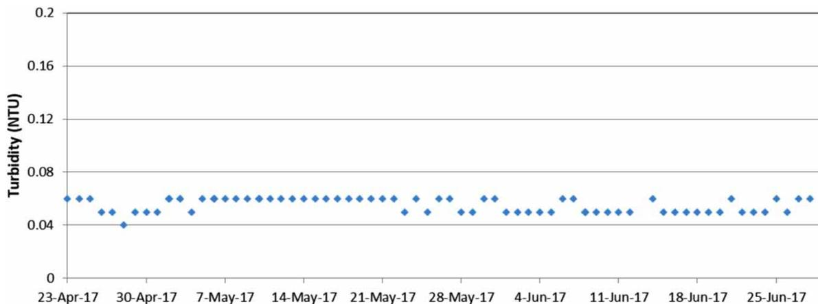
**Figure 6** | Permeate turbidity in Tank A.
