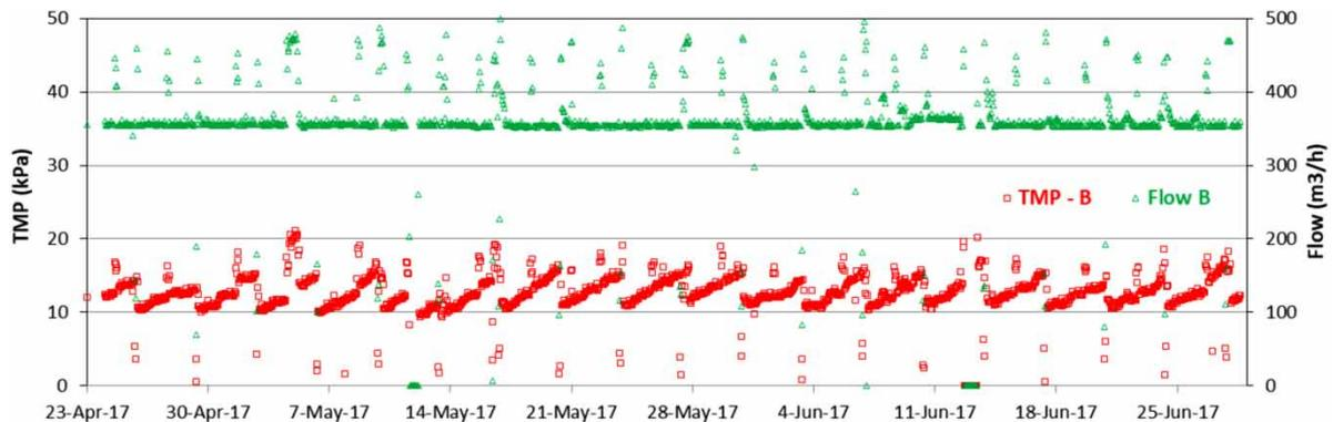
Figure 3 | Trend of TMP and permeate flow of Tank B.
