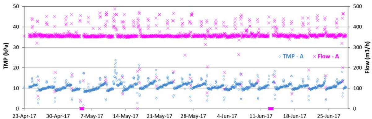
**Figure 2** | Trend of TMP and permeate flow of Tank A.
