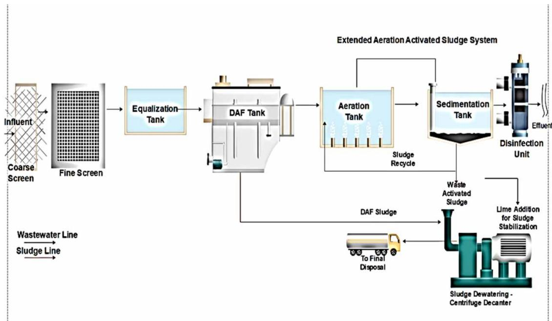
**Figure 1** | Available wastewater treatment process flow diagram.
