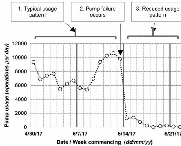
**Figure 6** | Pump failure event on India MkII hand pump in Mbankan, The Gambia.
