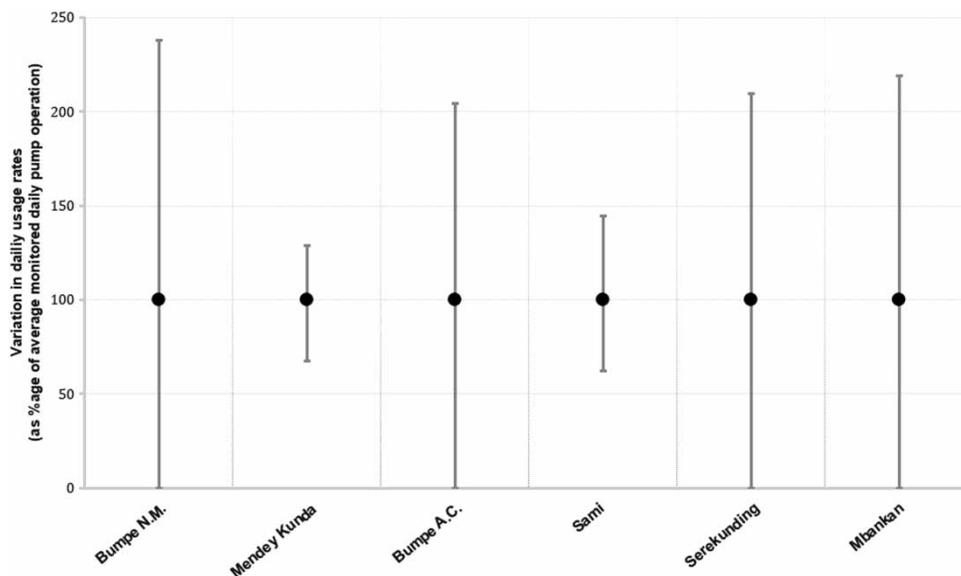
**Figure 7** | Operational ranges for six hand pumps in Gambia and Sierra Leone.
