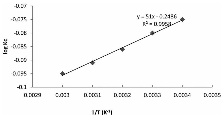
**Figure 5** | Graph of  $\log K_c$  vs.  $1/T$  showing effect of temperature change on Diresul Black's adsorption on alumina: adsorbent concentration 1 g; dye concentration 0.0124 M; contact time 20 min.
