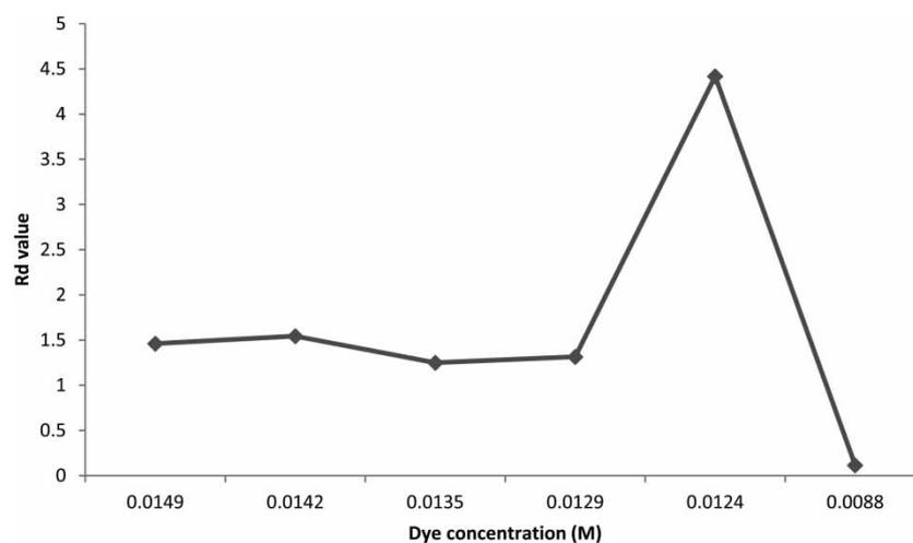
**Figure 3** | Effect of dye concentration on  $R_d$  value for adsorption of Diresul Black on alumina: temperature = 29 °C; adsorbent amount = 1 g; contact time = 20 min.
