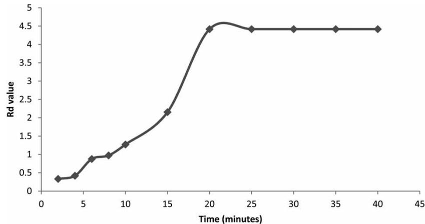
**Figure 2** | Effect of contact time on  $R_d$  value for Diresul Black's adsorption on alumina: temperature = 29 °C; dye concentration = 0.0124 M; adsorbent amount = 1 g.
