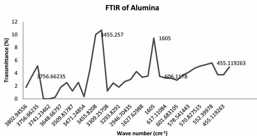
**Figure 1** | FTIR spectrum of alumina.
