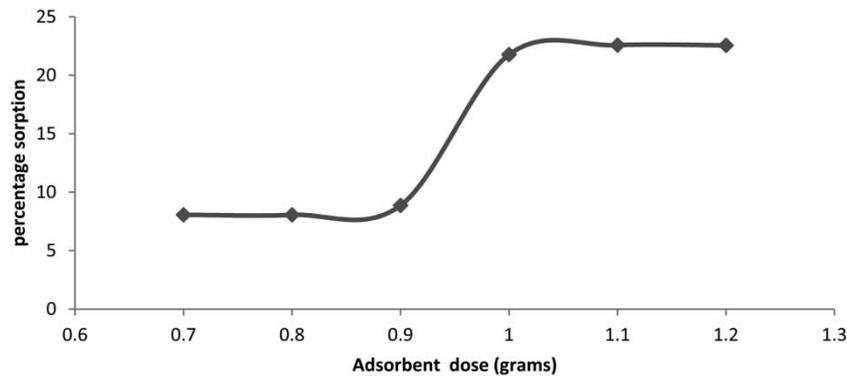
**Figure 4** | Effect of adsorbent amount on percentage sorption of Diresul Black on alumina: temperature 29 °C; dye concentration 0.0124 M; contact time 20 min.
