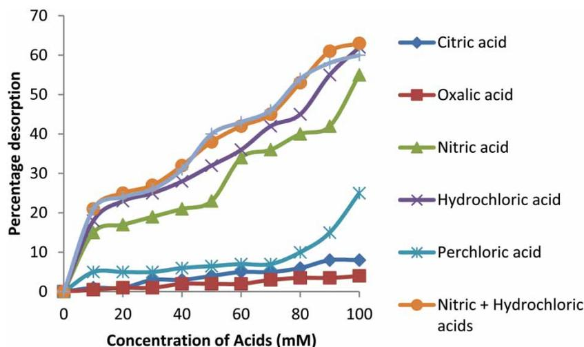
**Figure 8** | The desorption percentage of Diresul black from alumina by addition of different concentrations of various acids and acid combinations.
