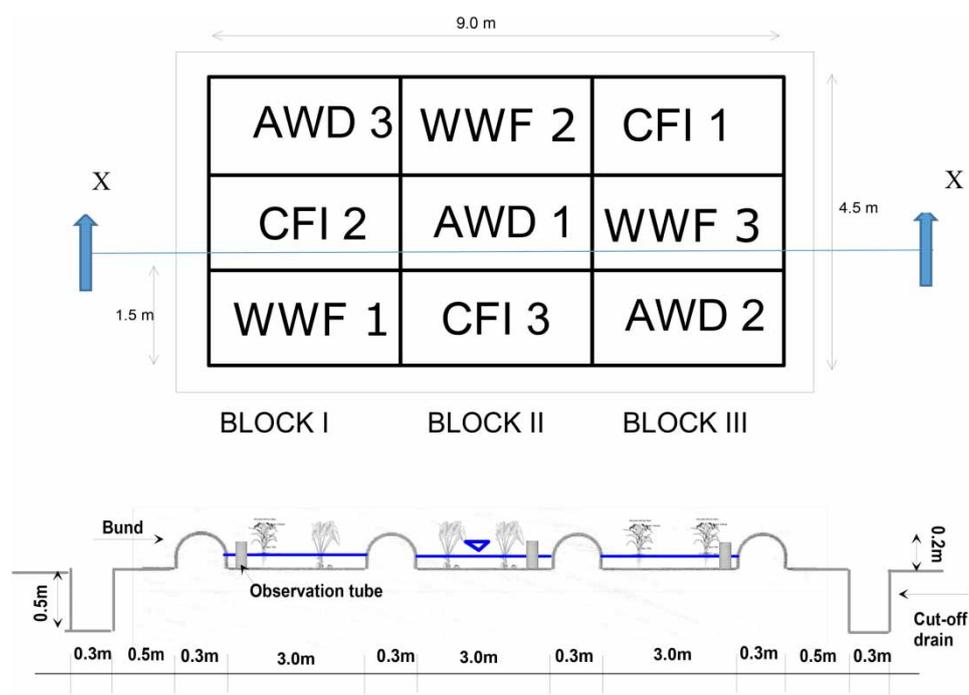
**Figure 2** | Field layout and cross-section X – X
