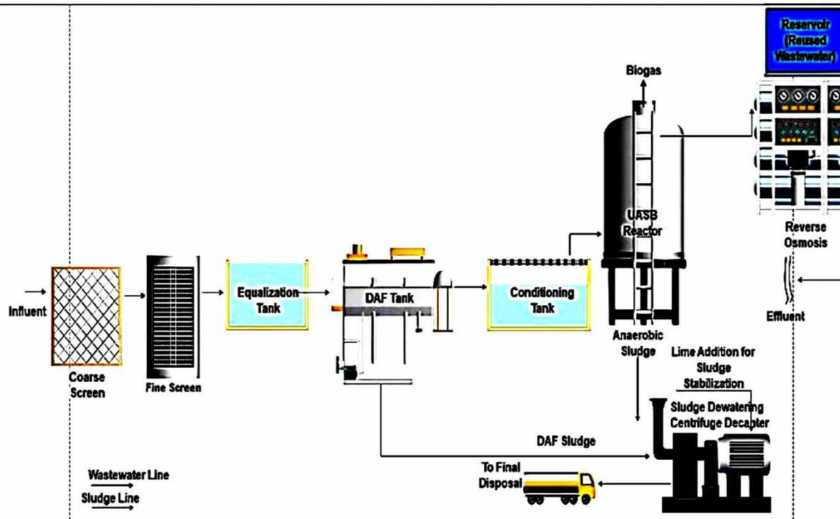
**Figure 1** | Current wastewater treatment process flow diagram.
