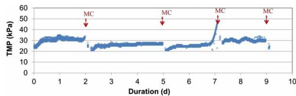
**Figure 8** | TMP trend of run-C (249 LMH) in the seawater pretreatment pilot system.
