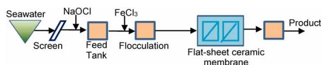
**Figure 3** | Schematic diagram of the seawater pretreatment pilot system.
