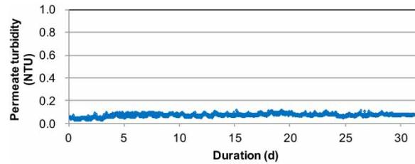
**Figure 10** | Permeate turbidity during run-B condition in the seawater pretreatment pilot system.
