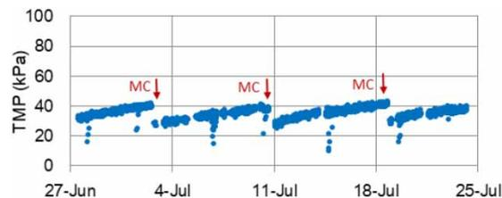
**Figure 4** | TMP trend for the ceramic membrane train in CAWW.
