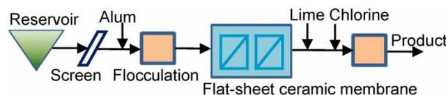
**Figure 1** | Schematic flow diagram of water treatment in CAWW.
