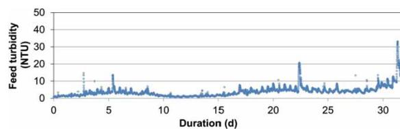
**Figure 9** | Feed turbidity during run-B condition in the seawater pretreatment pilot system.
