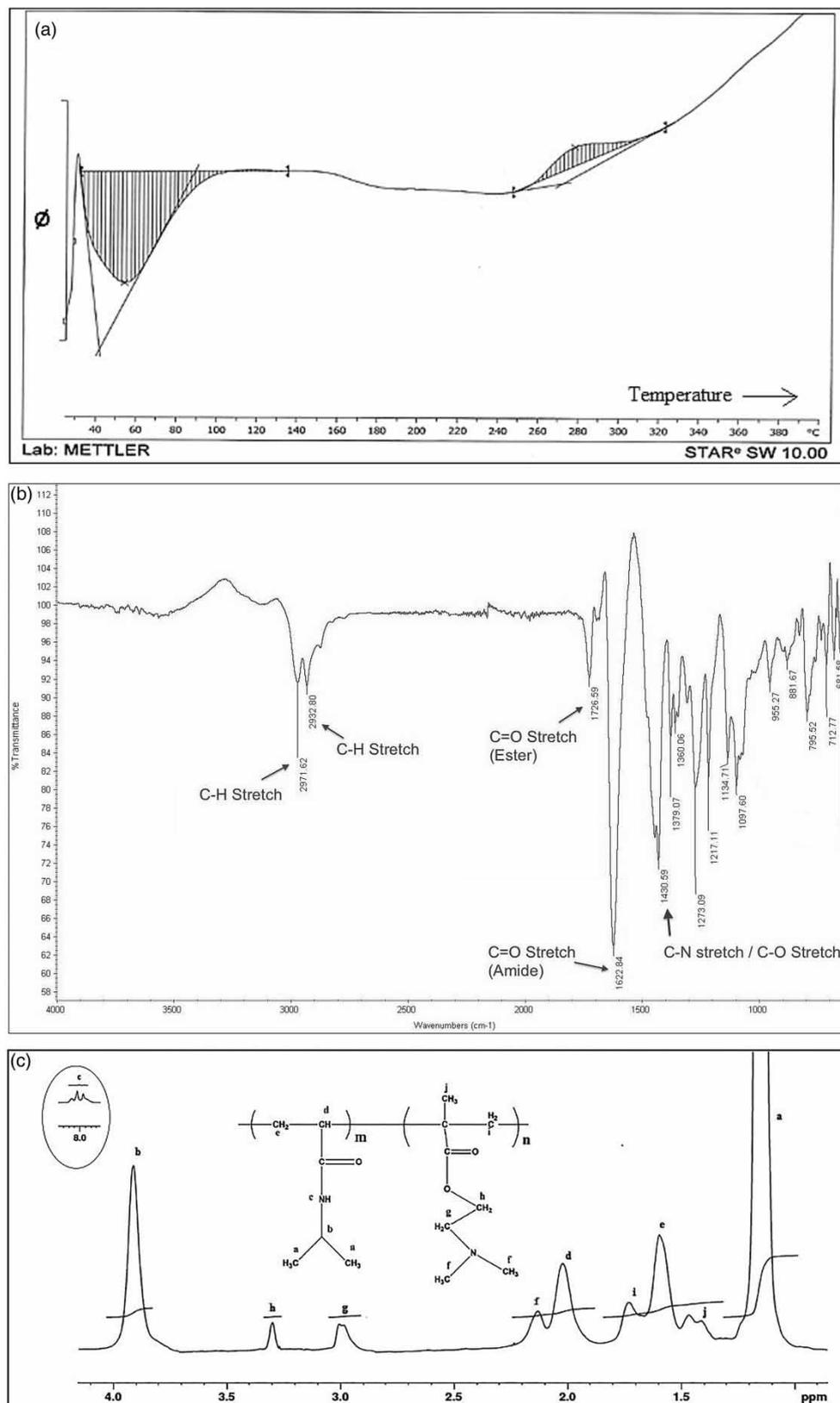
**Figure 2** | (a) DSC thermogram for CoP-1 (b) FT-IR spectrum of CoP-1 (c) <sup>1</sup>H-NMR spectrum of CoP-1.
