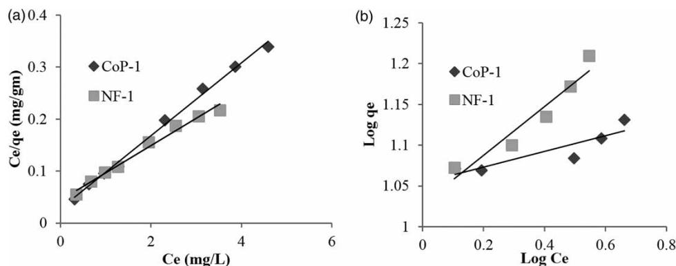
**Figure 5** | Dye adsorption isotherm model onto copolymer and nanofiber substrates. (a) Langmuir and (b) Freundlich.
