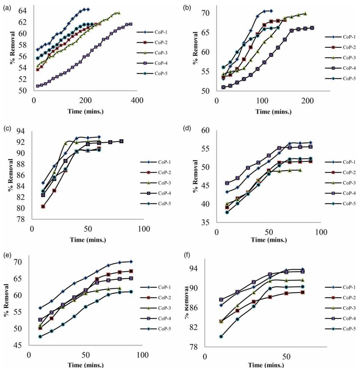
**Figure 4** | Optimization of equilibrium contact time for maximum adsorption by various co-polymers at concentrations and responsive conditions as: (a) 1 mg/ml at LCST (b) 2 mg/ml at LCST (c) 4 mg/ml at LCST (d) 1 mg/ml at pH cloud point (e) 2 mg/ml at pH cloud point (f) 4 mg/ml at pH cloud point. (Values are with mean  $\pm$  s.d. of 0.95–1.66).
