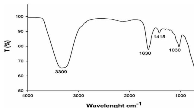
**Figure 2** | FTIR spectra of alginate-clinoptilolite beads.
