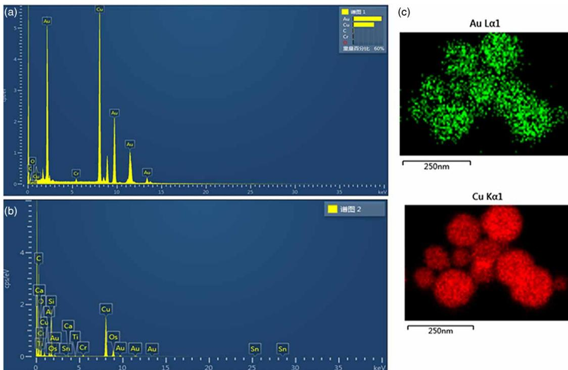
**Figure 4** | TEM-EDS of PVP-templated Au NPs acting on sewage (each sample was added to the copper mesh for testing).
