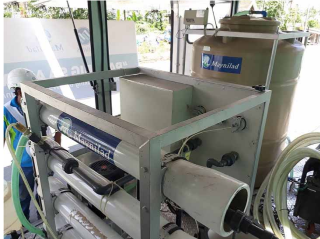
Figure 1 | Maynilad's mobile treatment plant, as deployed in disaster relief efforts after the Mayon volcano eruption, 2018.
