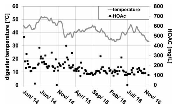
**Figure 12** | Organic acid concentration in digester of #WWTP\_A\_D1.
