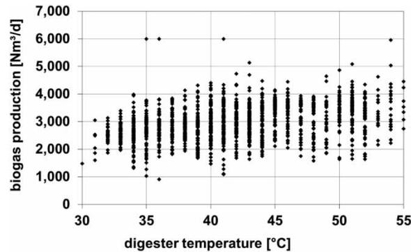
**Figure 5** | Relationship between biogas production and temperature for #WWTP\_A.
